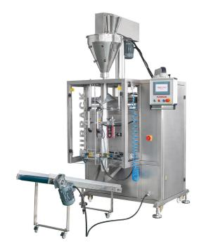
This machine can fill all kinds of non-flowing products such as, spices, coffee, cream, milk powder, pepper, chilli powder, vanilla etc. Product weight is adjusted by precious screw. The screw-pipe is used in different diameters for varying weights.
