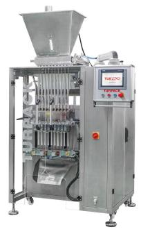
This machine is designed to fill free flowing products such as sugar, salt, spices and black pepper through volumetric cups into affixed three side sealed stickpack. The volume of the product feed into the volumetric containers can be adjusted between a curtain weight ranges, this assures that the desired weight is sensitively filled into the stickpack.
