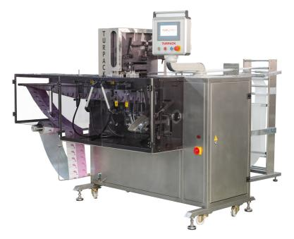
Single sachet wet wipes machine is used to pack single use wet tissues into a 4 side sealed sachet. it can do the work of folding, cutting, bag-forming, water-adding, slicing, code-printing and counting. Fully stainless steel construction.
