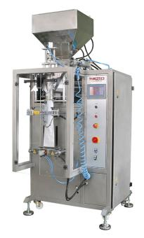
TP L-101 liquid packaging machine is most suitable for packing liquid products such as (Milk, Flavored Milk, Lassi, Curd, Juice Drinks, Water) with a servo motor dosing unit and pneumatic parts FESTO this machine offers high performance and accurate weights.
