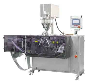
Horizontal machines are fully automatic machines and make 4 side sealed sachettype packages to fill powdery products. This machine can fill coffee, mix flour, powdered beverages, powder spices like cinnamon, black pepper, mixed spices, milk powder and powder chemicals, cosmetics and medicines. The sachet size is flexible, both width and height of the sachets can be changed depending on demand this gives the customer a flexible usage.
