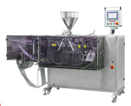
Horizontal Liquid Filling Machines allow fluid and dense liquids to be packed as the desired milli-grams into disposable sachets which are filled and sealed as 4 Sides Sachets. The fully automatic horizontal liquid filling machines are the most suitable solutions for food packing, especially cosmetics, chemistry, medicine, cleaning and so on .. The sachet widths are flexible. Both the width and height of the sachets can be changed depending on demand, this gives the customer a flexible
