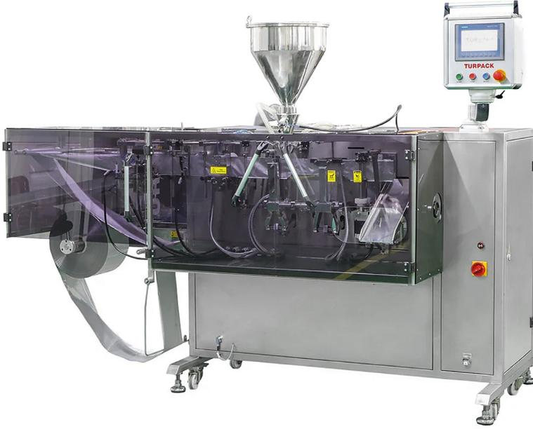
Horizontal packaging machine is fully automatic and prepare 4 side sealed sachet-type packages to fill free flowing granular products like sugar, salt, spices like free flow black pepper and other medicine, chemistry, cosmetics grained granules can be packaged trough precise volumetric cups using this model. The sachet size is flexible, both width and height of the sachets can be changed depending on demand this gives the customer a flexible usage.
