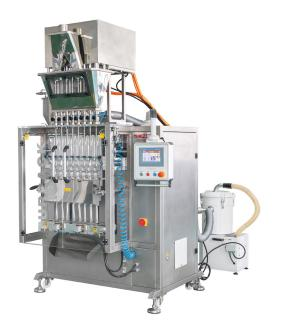
This fully automatic filling machine is designed to pack untouched, affixed-on-three-sides packets like coffee, coffee cream, energy drinks, medical powder that has no spontaneous fluency through screws by disposable products. Non free flowing powder products can be packaged with this machine using screws synchronized with PLC in a high level of sensitivity. The machine can produce 100 pcs/min using 3 channels and 350 pcs/min using 10 channels.
