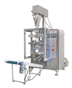
This fully automatic packaging machine that is designed to prepare 4 side sealed sachet-type packages, and to place untouched non free flowing powdered products. Cream, coffee, mix flour, powdered beverages, black pepper, powder, cinnamon, soups, yeast, milk powder and similar products that have no self fluidity can be packed with a servo motor driven dosing system to assure precise weights in each packet. The machine can produce 60 pcs/min using 2 channels and 240 pieces with 8 channels.
