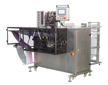
Single sachet wet wipes machine is used to pack single use wet tissues into a 4 side sealed sachet. it can do the work of folding, cutting, bagforming, water-adding, slicing, codeprinting and counting. Fully stainless steel construction.
