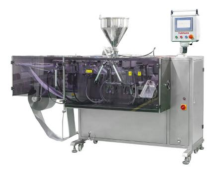
Horizontal Liquid Filling Machines allow fluid and dense liquids to be packed as the desired milli-grams into disposable sachets which are filled and sealed as 4 Sides Sachets. The fully automatic horizontal liquid filling machines are the most suitable solutions for food packing, especially cosmetics, chemistry, medicine, cleaning and so on .. The sachet widths are flexible. Both the width and height of the sachets can be changed depending on demand, this gives the customer a flexible usage.
