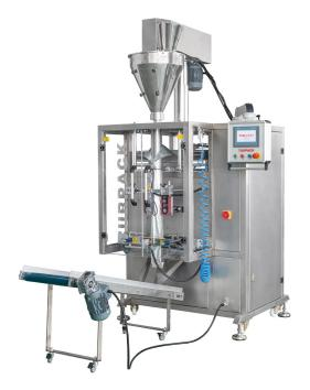
This machine can fill all kinds of nonflowing products such as, spices, coffee, cream, milk powder, pepper, chilli powder, vanilla etc. Product weight is adjusted by precious screw. The screw-pipe is used in different diameters for varying weights.
